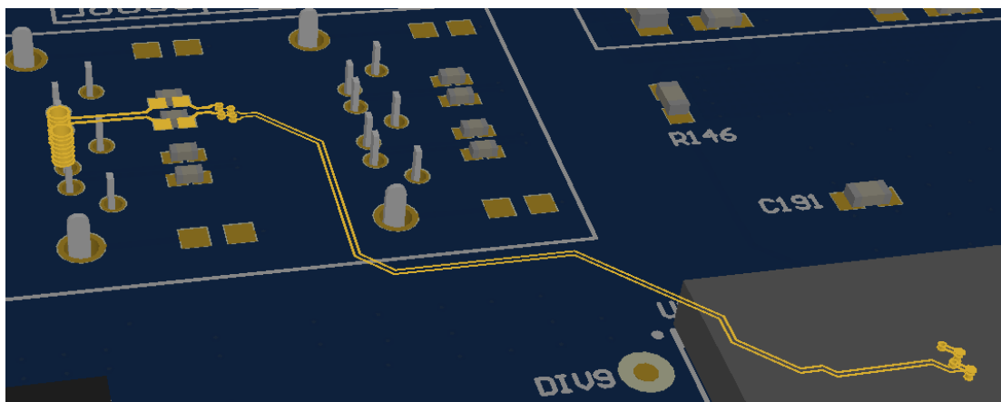
Figure 6.6: Analysed SATA traces, SATA_RX2
