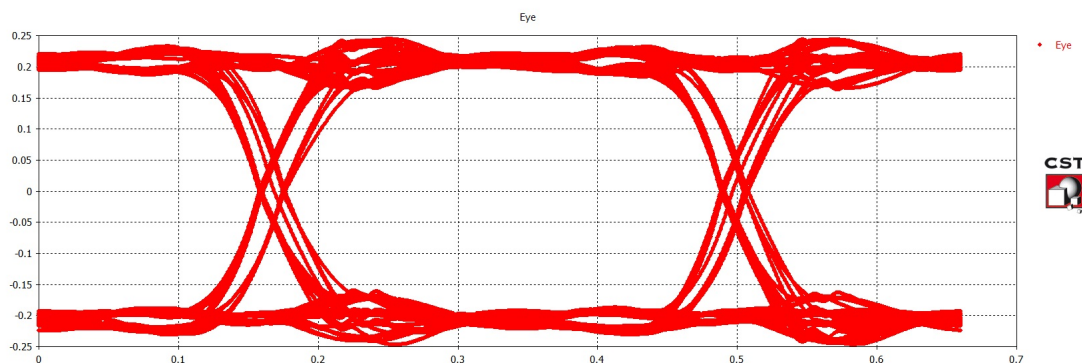
Figure 6.9: Simulated eye diagram using SATA 3 Gbit s -1 standard signal setup
